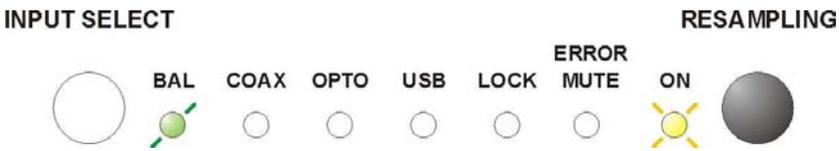
**1st Menu item: Sharp or soft digital filter in the D/A converter**
