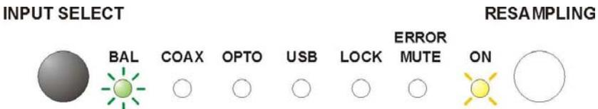
LED off = the digital filter has sharp roll-off (ex works setting)
